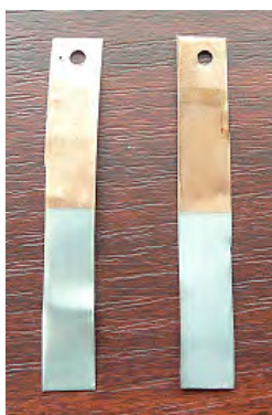
Figure 1. Sn deposit onto Cu substrate from choline chloride based ionic liquids containing \text{SnCl}_2
