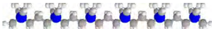
Fig. 1: Schematic representation of the portion of 3-3 ionene polymer; dark circles – N atoms, grey – C atoms, white – H atoms.
